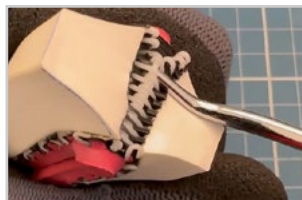
Pry up the pin using a pick
