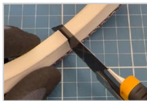
Cut the V-guide down to the mesh
