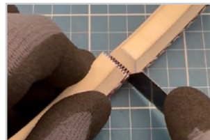
Carefully cut the coating of the belt
